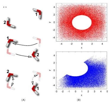
Fig. 1. Panel A shows the relabeling step for one pair of water molecules. In panel B the compacting of the configuration space density is illustrated for the 2D case.
