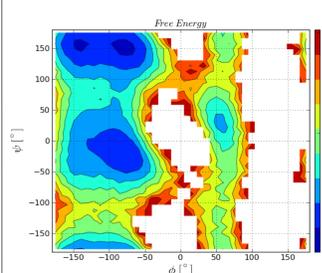
The simulations were done in the AMBER99SB forcefield, using the GROMACS work package with its implicit solvent implementation. To restrict a single simulation to a certain subspace, we used PLUMED<sup>[2]</sup> to add a rmsd-based potential.
