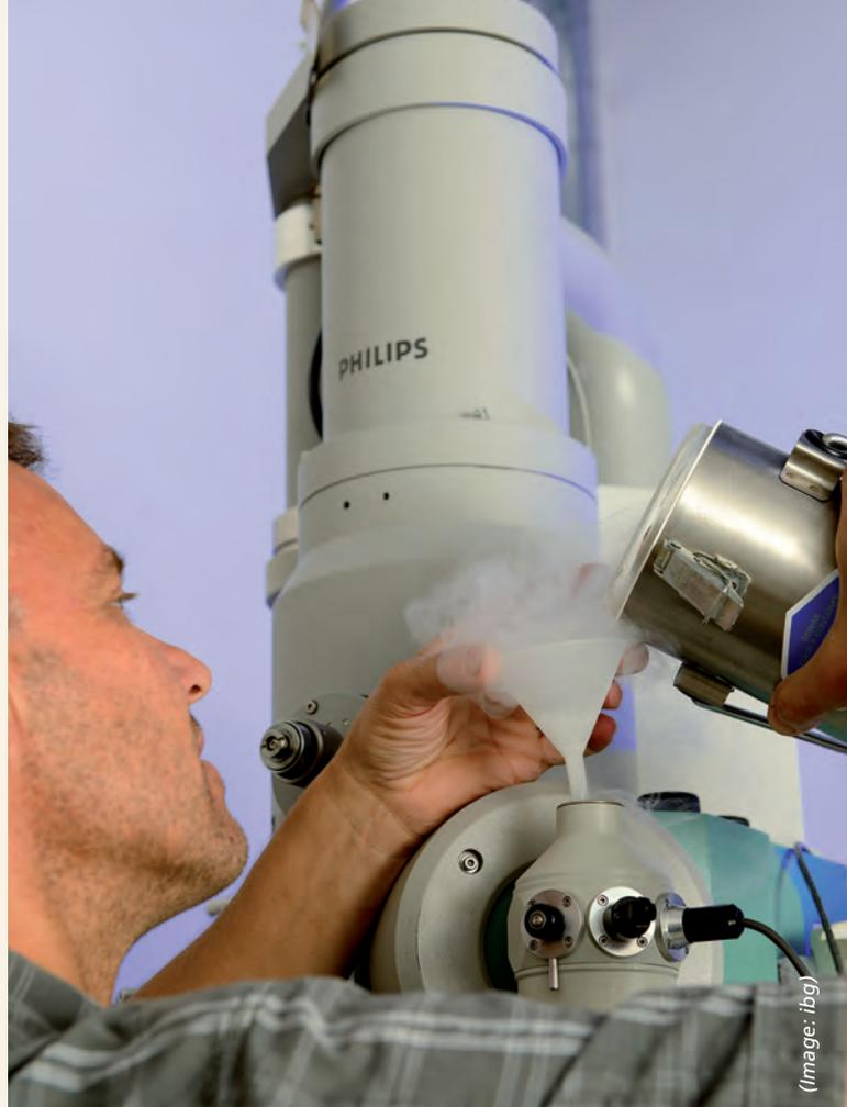
Dietmar Riedel pours liquid nitrogen into the dewar vessel to cool down the microscope.
